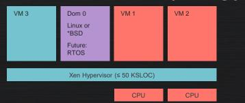
Dom0less VMs loaded by uBoot and booted by Xen (not Dom0), pinned to a CPU via the Null scheduler and I/O handled by device assignment
